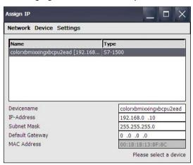
To identify the selected device in the plant, you can use the "Device > Flash" function. The "Flash" function causes the display of the selected HMI device or the "RUN/STOP" LED of a controller to flash.
